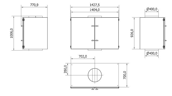
Cabinet for compact filter type AF-A1 (excl. filters) with connection in through bottom and out of top:
