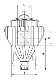
Jet filter type QFG-A (max. 5,000Pa):
