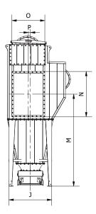
Jet filter type QFG-A (max. 5,000Pa): ATEX zone: 21/22
