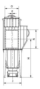
Jet filter type QFG-A (max. 5,000Pa): ATEX zone: 21/21
