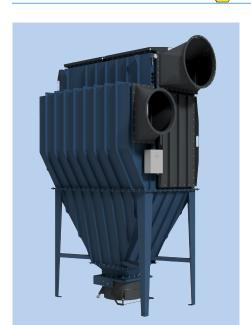
Energy-efficient unit for larger filtration tasks. Suitable for filtration of grinding dust, blasting media dust, cutting fumes and dusty air containing metal, rock, plastic etc. or from handling various powder mixes. Unit is constructed for application at ATEX-zones 21-22 and is standard equipped with relief membrane, designed to break at an explosion, whereby the unit is relieved and explosions controlled.
