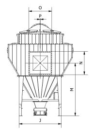
Jet filter type QFG-A (max. 5,000Pa): ATEX zone: 21/22
