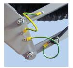
Bend buttom with earth cable connections to parallelogram.
