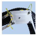
Joint Intermediate plates at top joint with relief cables between construction parts.
