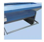
Foot pedal With easy/light pressure on foot pedal, the clamp plate is lifted.
