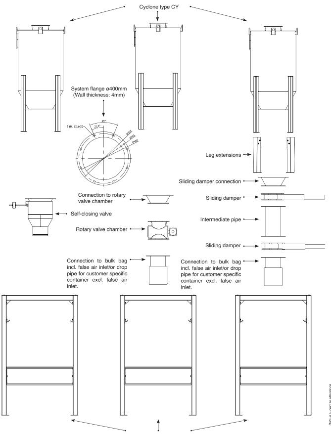
Underframe for suspension of bulk bag or insertion of customer specific container.
