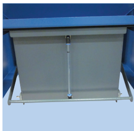
Water bath Water bath is easily removed and subsequently serviced.
