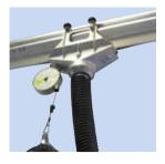
**Exhaust channel**Spring balancer used in connection with exhaust channel.
