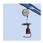
**Tool**Balancer used for the suspension of tools that are often used.
